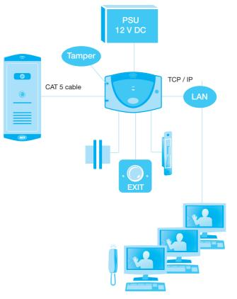
Up to 25 PC's running VIP software with PC handsets connected.
